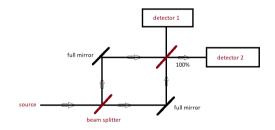
We modify the experiment by adding a second beam splitter and two fully reflecting mirrors. In this modified set-up the result is non-intuitive. The photons do not hit each detector with a 50% chance.
